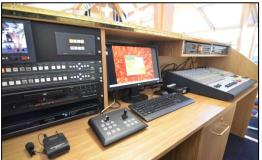
A bespoke AV console designed specifically for the Church contains all control hardware including an Allen & Heath GL2400 mixer, AV optimised PC, dual Kramer Switching-scaler, Datavideo preview screen and rec/playback decks.
